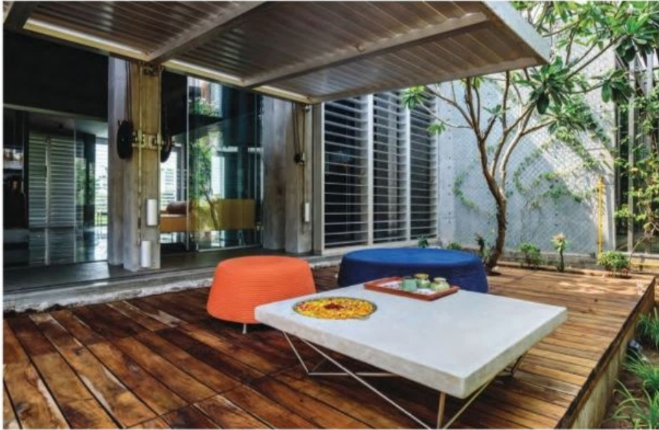
1 These louvers can also be lifted up, much like a bird's wingspan, to create a pergola.
